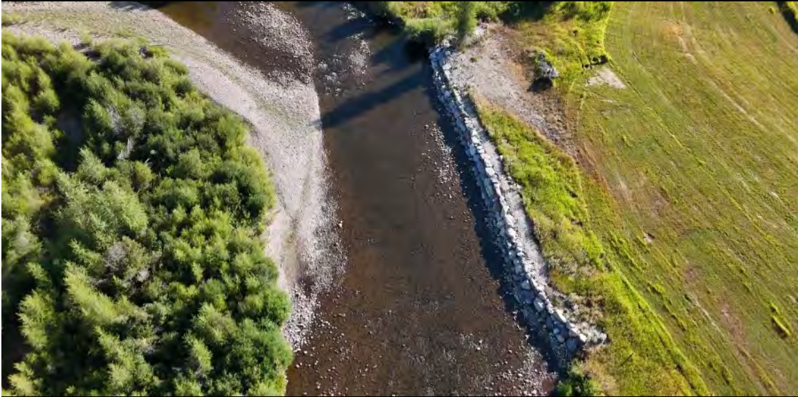
Figure A-28. Example of modified riverbank and floodplain (right) opposite a relatively intact, natural channel and floodplain (left) in riverscape 10. “Pairings” like this, where one bank is extensively modified through human actions while the opposite retains a relatively natural character, are common throughout the Elk River segment.
